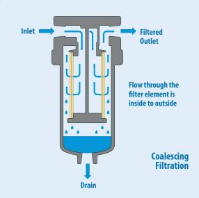
Coalescing filters can be seen as multifunctional filtration solutions thanks to their ability to filter particulates just as efficiently as they coalesce aerosols and droplets. Meaning, if you have an application that requires both types of filtration, a coalescing filter is ideal.
