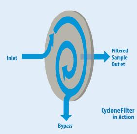
Due to this cyclone effect, the filter disc is kept clean for a long period of time, extending the period required between service intervals when compared to standard filters.
