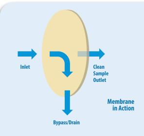
The effective combination of carefully manufactured components prevents 100% of liquid molecules from flowing through the membrane; allowing only molecules of gas to pass. Any liquid removed flows through to the drain port. This port can also be used as a bypass function for the main flow.
