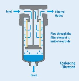
Coalescing filters can be seen as multifunctional filtration solutions thanks to their ability to filter particulates just as efficiently as they coalesce aerosols and droplets. Meaning, if you have an application that requires both types of filtration, a coalescing filter is ideal.
