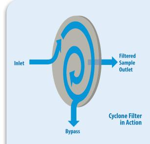
Due to this cyclone effect, the filter disc is kept clean for a long period of time, extending the period required between service intervals when compared to standard filters.
